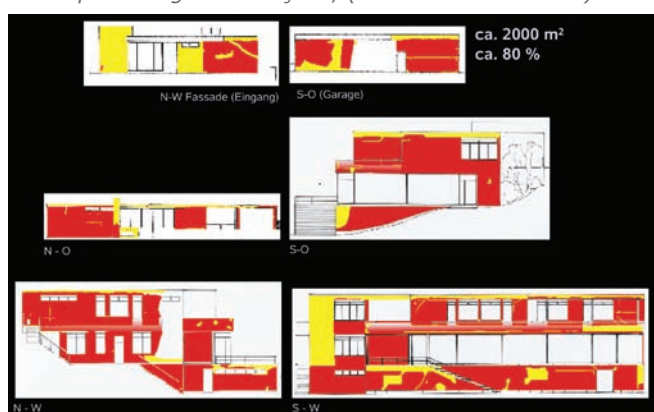
15. Brno (Czech Republic), Tugendhat House 1930, Ludwig Mies van der Rohe. Mapping of the extent of the preservation of the plastering of the façade, (Source : HAWK 2004)
