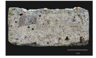
Peine, Lessing Loge, east facade, stone plaster / sample: Both pictures show large paneled gypsum crystals. Photo: Meinhard-Degen, 2007.
