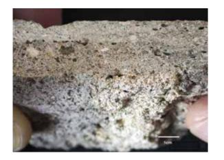
Peine, Lessing Lodge, cast stone plaster: sample / transversal layer in angled light / daylight with flushmounted and adhering plaster. Photo: HAWK / Götz, 2007.
