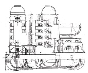
(left) Potsdam, Telegrafenberg, Einstein Tower 1920-1922, Architect Erich Mendelsohn. Mapping of the mixed construction Red: brickwork, green: reinforced concrete. Graphics, Huse 2000, p.93. Gerhard Pichler.
