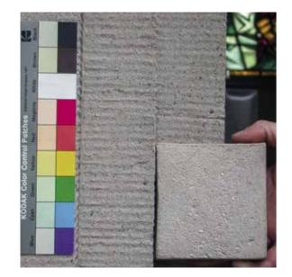
Repair mortar we assembled in comparison with the construction concrete block at the stucco border of the entrance area. Photo: HAWK / Götz, 2007.
