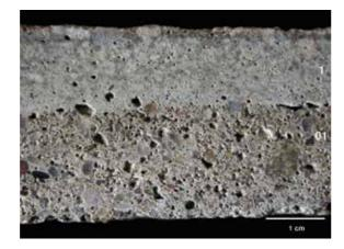
Cast stone plaster: sample / transverse layer in angled light / daylight. Photo: HAWK / Götz 2007.
